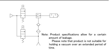
2) Prevention of reverse flow to vacuum source (simple vacuum holding)
