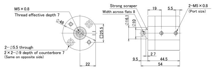
Note 1: Since this product has no built-in magnet, positions cannot be detected by auto switches.
