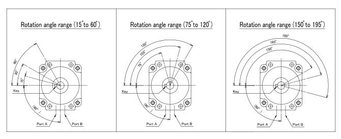
The illustrations above show the key positions when B port is pressurized.
