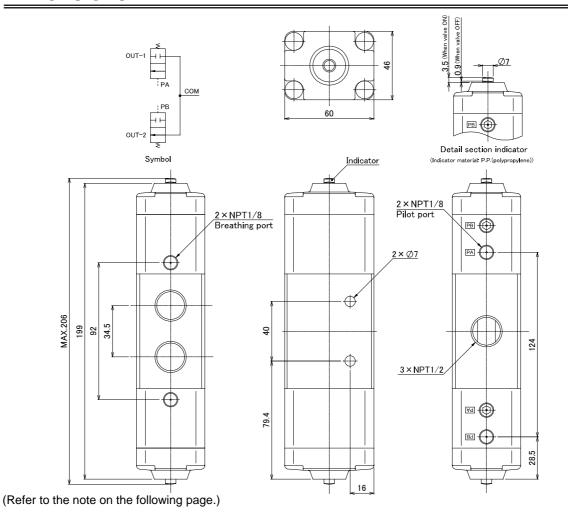
Note: This product is assembled and packaged in a clean room in the same way as standard product of Series LV. Refer to "Series LV Quality Process Diagram" in "High Purity Chemical Valve" catalog (CAT.ES70-16B) for details.
