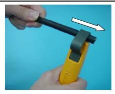
(2) Slide the tool longitudinally to cut into the outer layer (Note 1).
