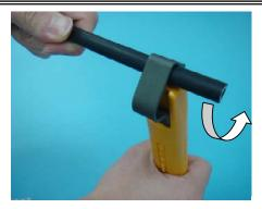
(1) Rotate the tool circumferentially to cut into the outer layer (Note 1).
