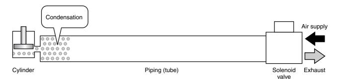
From observation of the above, one can see that condensation is largely influenced by the volume of the cylinder and piping.
