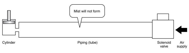
Note) Most piping is usually long, with a larger volume than the cylinder volume. Therefore, the piping is larger than the cylinder in the above figure.
