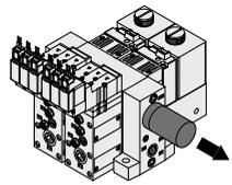
If there are a large number of ejectors that are linked on a manifold and operate simultaneously, use the built-in silencer type or the port exhaust type.
