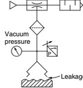
If a considerable amount of leakage occurs between the workpiece and the pad, resulting in incomplete adsorption, or to shorten the adsorption and transfer time, select an ejector nozzle with a larger diameter from the ZH, ZR, or ZL series.
