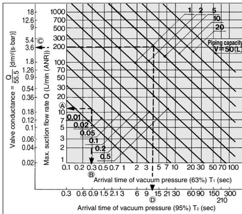
\* Conversely, the size of the ejector or the size of the switching valve of the vacuum pump system can be obtained from the adsorption response time.
