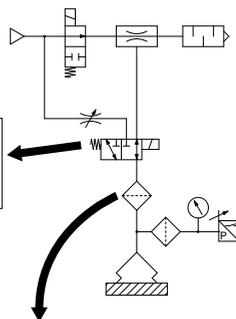
For the release valve, select a 2/3 port valve with a low vacuum specification. Also, use a needle valve to regulate the release flow rate.
