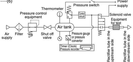
Fig. (2) Test circuit based on JIS B 8390: 2000
