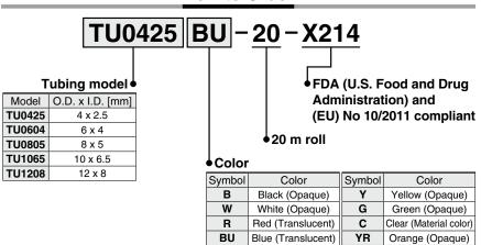
\* Note that the model number is not printed on the tube body.
