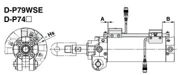
\* The above drawing is the switch rod mounting example for the D-P79WSE.
