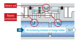
\* There is no bypass construction for the 1 and 2 L ranges.
