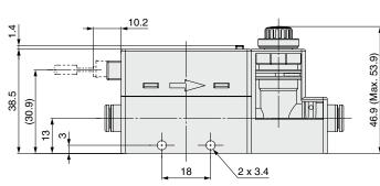
[mm] Model Α PF2M705/710S-C4(-L) 87.1 ø2.8 depth 8.4 ø2.5 depth 6 PF2M705/710/725/750S 87.9 ø2.8 depth 8.4 ø2.5 depth 6 -C6(-L) PF2M725/750S-N7(-L) 95.5 ø2.8 depth 8.4 ø2.5 depth 6 PF2M711/721S-C8(-L) 96 ø2.8 depth 6.2 ø2.5 depth 5 PF2M711/721S-N7(-L) 92.6 ø2.8 depth 6.2 ø2.5 depth 5
