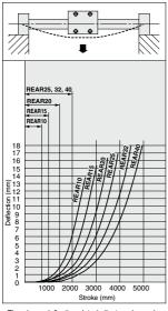
\*The above deflection data indicate values when the external slider has moved to the middle of the stroke.
