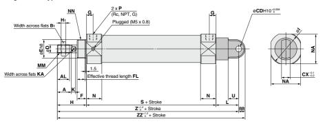
(mm) Bore (mm) Α ΑL В1 CD СХ D Ε F FL G н Нı 1 Κ KA L ММ N 20\_0,033 20 18 15.5 13 9 10 8 13 10.5 10 41 5 33.5 5 6 30 M8 x 1.25 20 22 19.5 17 9 10 10 26\_0.033 13 10.5 10 45 37.5 5.5 8 30 M10 x 1.25 20 25 6 26\_0.033 32 22 19.5 17 9 10 12 13 10.5 11 45 6 46.5 5.5 10 30 M10 x 1.25 22 32\_0,039 40 24 21 22 10 15 14 16 13.5 12.5 50 56.2 12 39 M14 x 1.5 26.5
