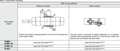
Note 2) Minimum stroke for auto switch mounting in types other than those mentioned in Note 1.
