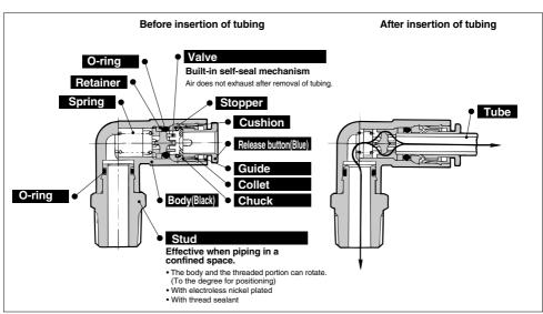
One-touch fitting (built-in self-seal mechanism) to prevent air exhaust when removing tube.
