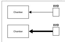
In the initial state, the sub-valve opens and the set amount (needle valve) is supplied slowly into the chamber.
