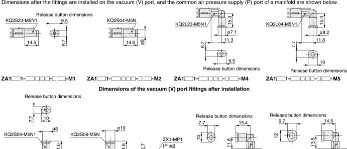
ZZA1 \_\_\_\_-\_3 Dimensions after the fittings are installed on the common air pressure supply (P) port
