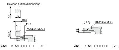
Dimensions of the air pressure supply (P) port fittings after installation
