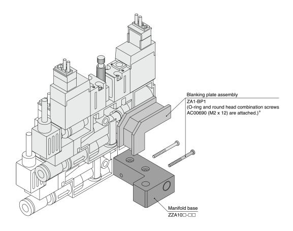
An assembly kit (part no. ZA1-OP-1) is available which includes 10 pcs each of O-rings and round head combination screws.
