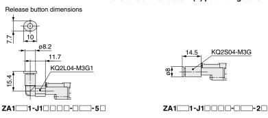
Dimensions of the air pressure supply (P) port fittings after installation
