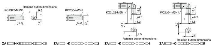
Dimensions of the vacuum (V) port fittings after installation
