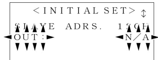
Figure 5-30 Initial Setting Screen 3: OUT
