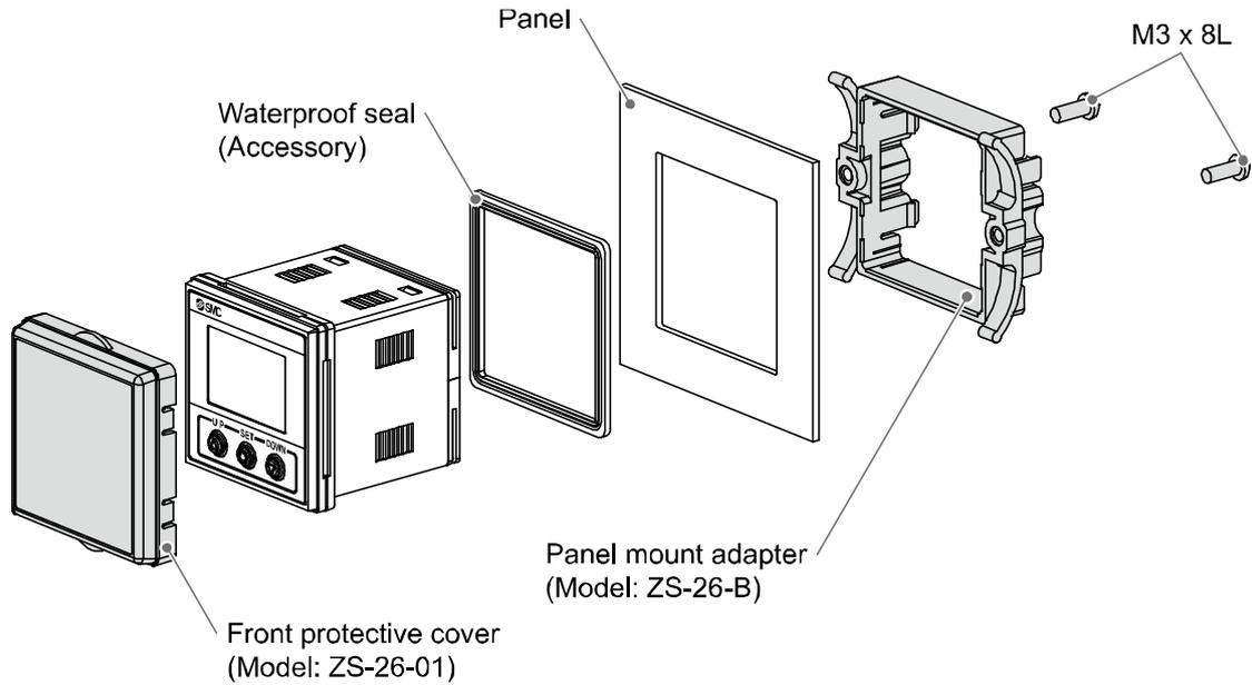
\*: The panel mount adapter can be rotated by 90 degrees for mounting.
