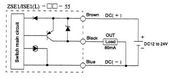
Brown lead: Connect to DC power (+) terminal to operate switch main circuit. Blue lead : Connect to power GND terminal.
