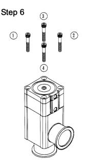
Tighten bolts in numerical order in above drawing. First, tighten them evenly by hand until just before O-ring is squeezed. Then, tighten them altogether.
