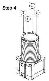
Apply ethanol to clean paper to wipe off dust on O-ring surface, and place the ring to O-ring groove. Press O-ring in numerical order in above drawing (press diagonally) to mount O-ring into the groove. gloves which (Put on generate no particle)
