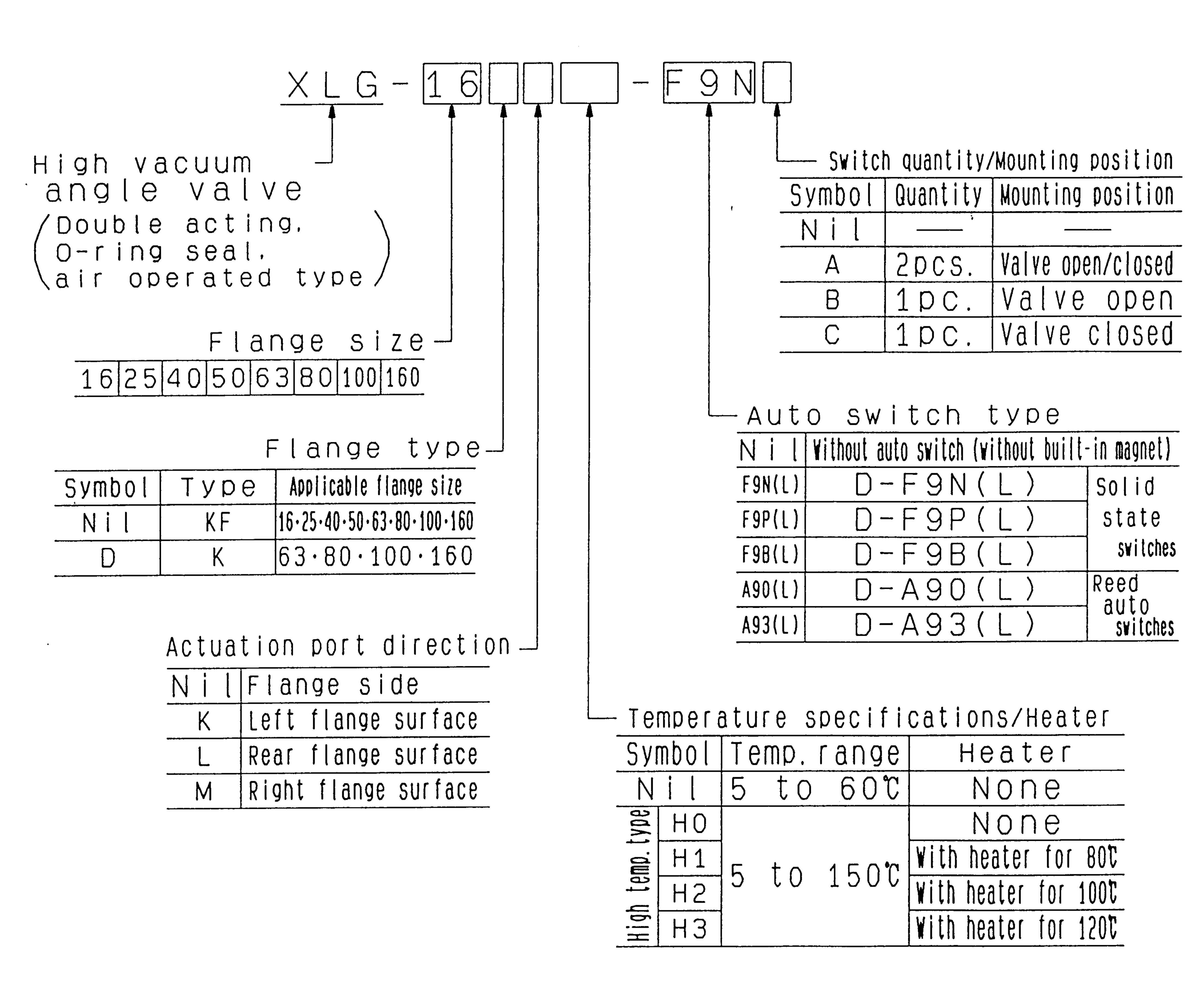
(Note)The combination of "with heater(H1, H2 and H3)" and "with auto-switch" is impossible.
