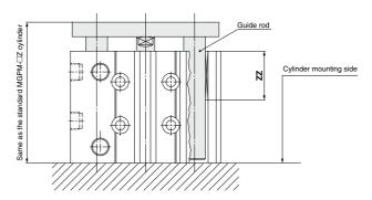
Note) The total length (ZZ) of the guide rod bushing is shorter than the standard type.
