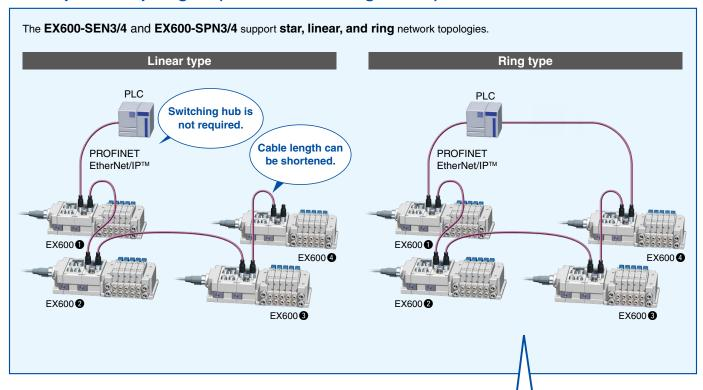
For ring networks, communication can be continued even if one of the communication cables in the network is disconnected or damaged. As the EX600-SEN3/4 supports Device Level Ring (DLR), and the EX600-SPN3/4 supports Media Redundancy Protocol (MRP), the disconnected point can be identified.
