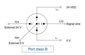
The control power supply wire, external power supply wire, and signal wire can be connected with one cable. (Mainly for actuators)
