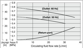
\* When the circulating fluid flow is below 6 L/min, the in-built operation stop alarm will be activated. It is not possible to run the equipment. (common for all models)
