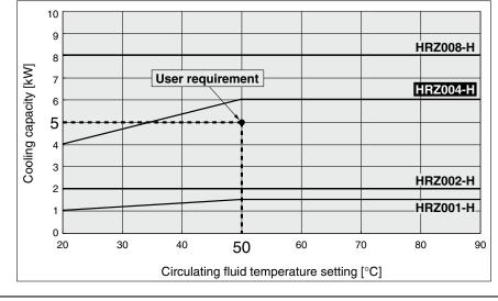
The point plotted in the graph is the requirement from the user. Select the thermo-chiller models exceeding this point. In this case, select the **HRZ004-H**.
