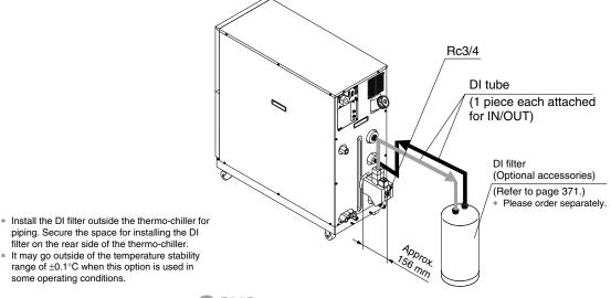
piping. Secure the space for installing the DI filter on the rear side of the thermo-chiller. It may go outside of the temperature stability
