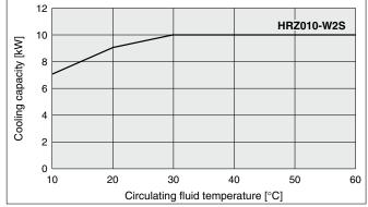
\* When pump inverter is operating at frequency of 60 Hz (maximum).
