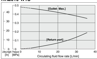
When the circulating fluid flow is below 6 L/min, the in-built operation stop alarm will be activated. It is not possible to run the equipment. (common for all models)
