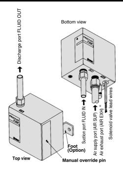
\* The PB1013 air operated type has a plug in the air exhaust port <AIR EXH>.
