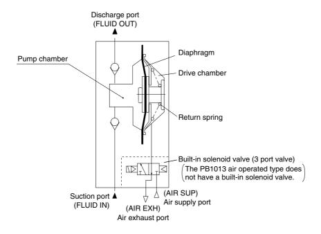
When air is supplied and the built-in solenoid valve is turned ON, air enters the drive chamber and the diaphragm moves to the left. Due to this movement, the fluid in the pump chamber passes through the upper check valve and is discharged to the OUT side.
