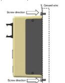
• DIN-rail mounting type (LECA6\*\*D-\*) installation onto the DIN rail
