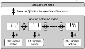
Press and hold the SET button for 2 seconds or longer in function selection mode to return to measurement mode.
