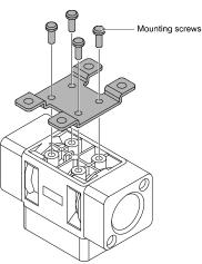
Mount the product with bracket using M4 screws (4 pcs.) or equivalent.
