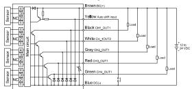
PSE201-(M)#: PNP open collector 5 outputs + Auto-shift 1 input Max. 80 mA. Residual voltage 1 V max.
