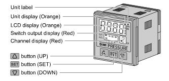
Switch output display (Red): ON when OUT1 (CH1 to CH4) and/or OUT2 (only CH1) is ON.
