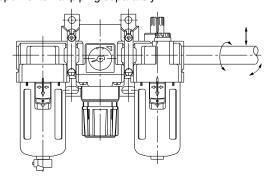
3. Piping materials without flexibility, such as steel tube piping, are prone to be affected by excess moment loads and vibrations from the piping side. Use flexible tubing in between to avoid such effects.
