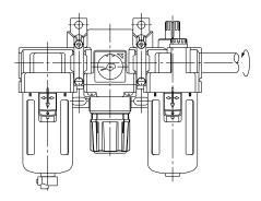
2. Avoid excessive torsional moment or bending moment other than those caused by the equipment's own weight, as this can cause damage.
